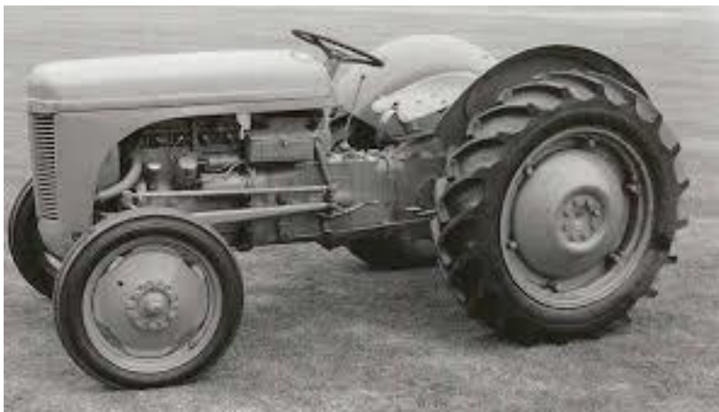
Harry Ferguson in 1949 introduced his now famous Ferguson tractor with its revolutionary 3 point linkage.
